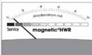
The meter needle is permanently near the red area and falls to "0" when the HWR plus is drained.
