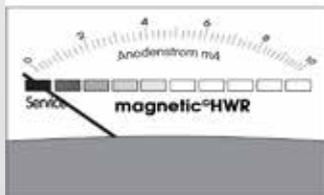
The meter needle falls completely into the red area some years after the commissioning.
