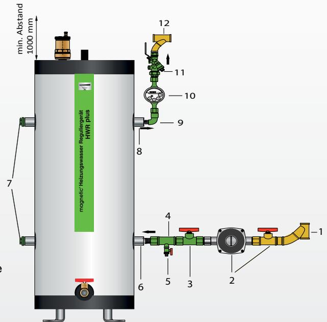
When installing the magnetic® HWR 50/100 plus as bypass, it is necessary to adjust the flow. It is possible to control and document flow by means of the water metre provided.
